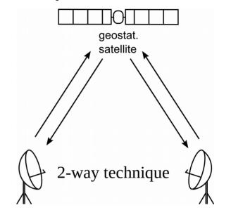
Instability depends significantly on signal properties set by the station (signal power, modulation bandwidth)
