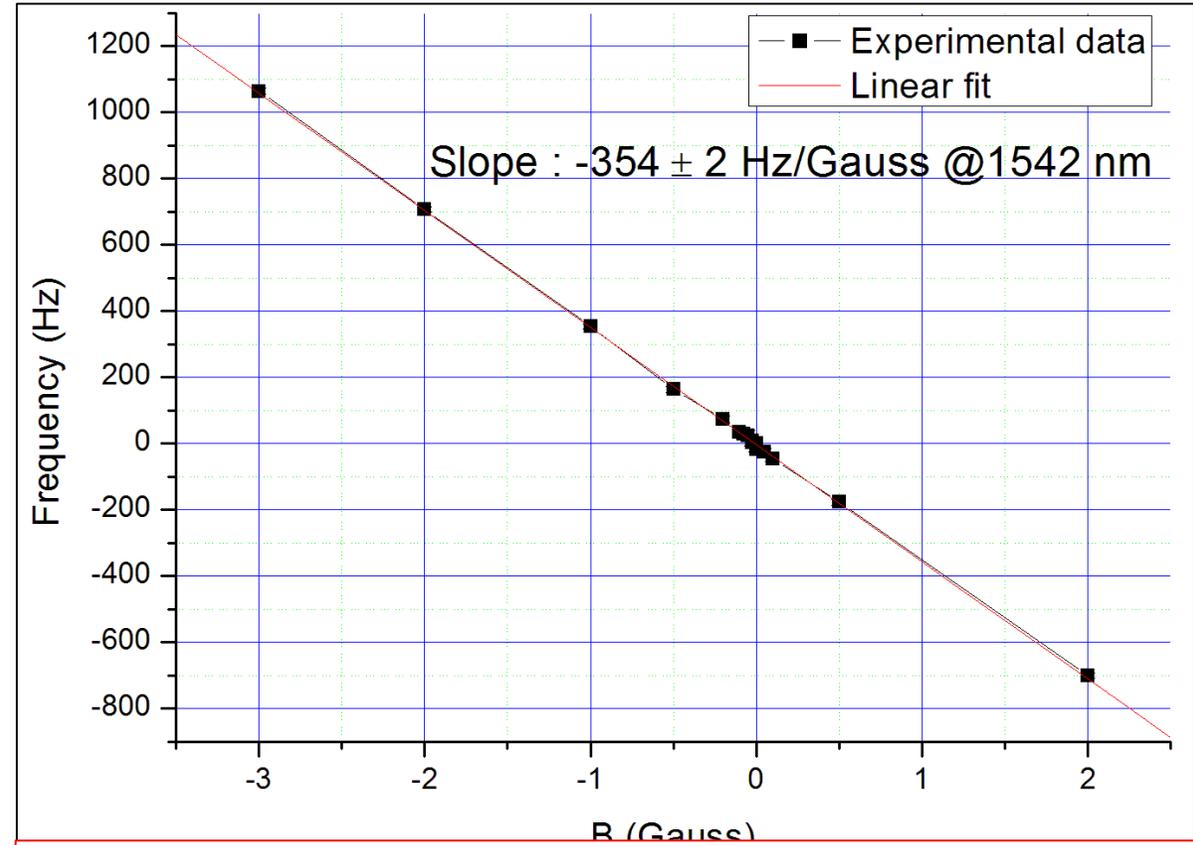
Frequency shift :  $\Delta \nu \sim 1 \text{ kHz / Gauss @ } 514.03 \text{ nm}$
