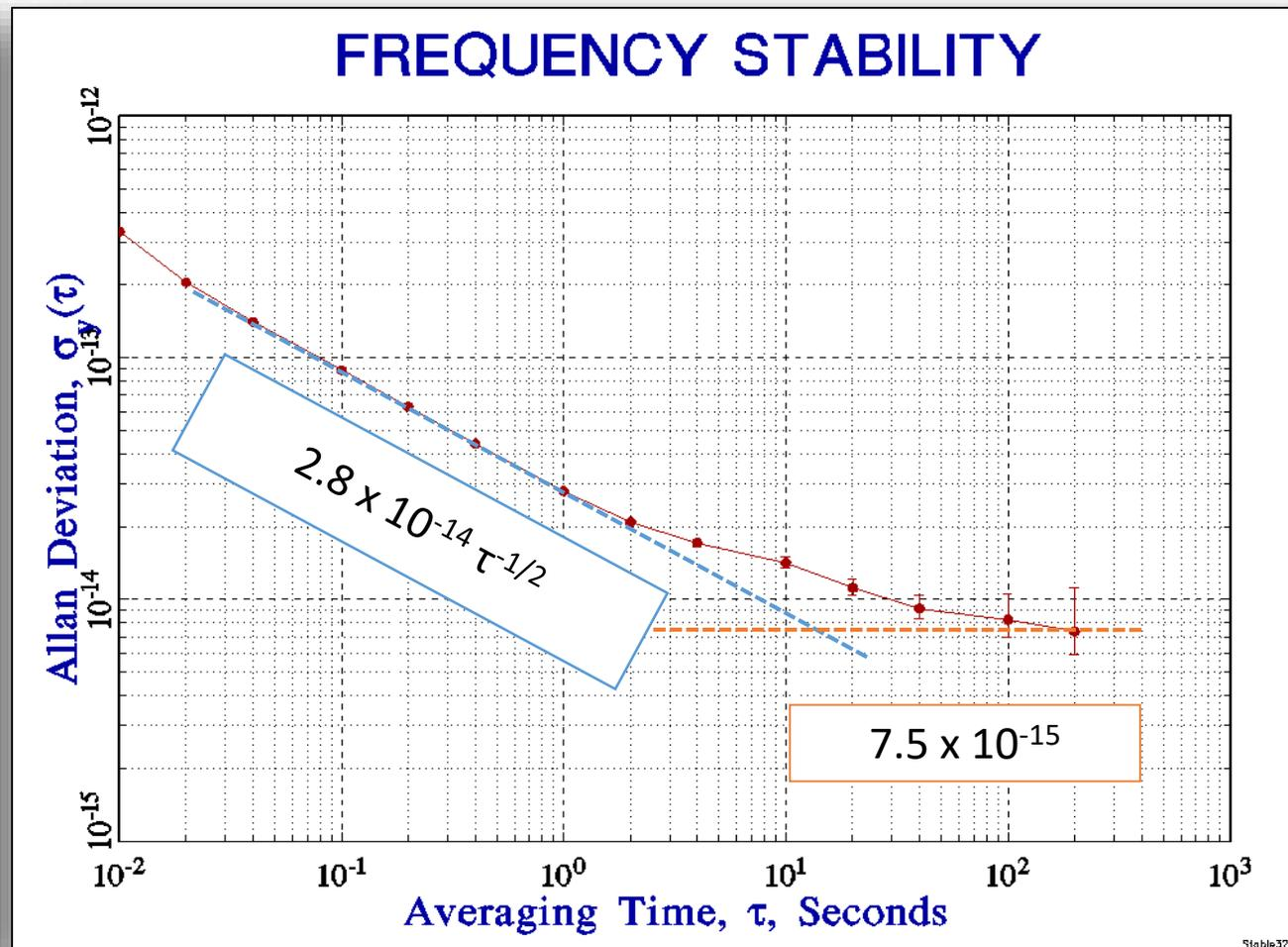
This long term frequency stability was obtained only during short period in the night when the **metro lines are stopped**
