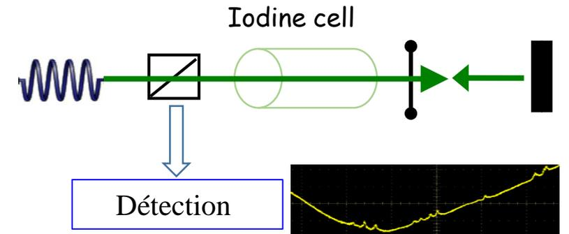
Third derivative of the iodine line is used to frequency stabilize the fiber laser
