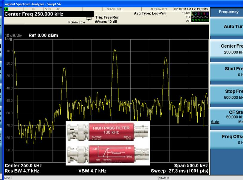
Photodiode output + homemade filters
