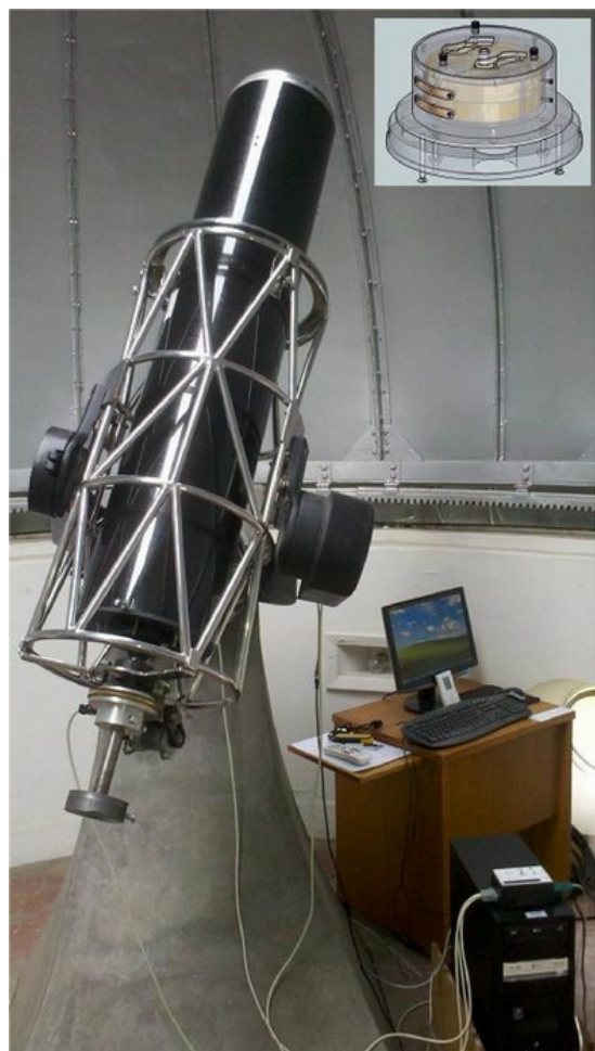
Figure 1: The Heliometer developed at Observatório Nacional/MCTI. The hemi-mirrors and containing cell are shown in the side detail.
