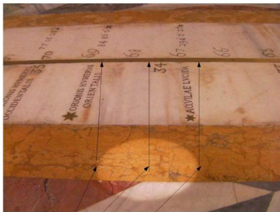
Figure 1: The image of the Sun is projected through a pinhole on the floor moving up on September 2 nd 2014.
