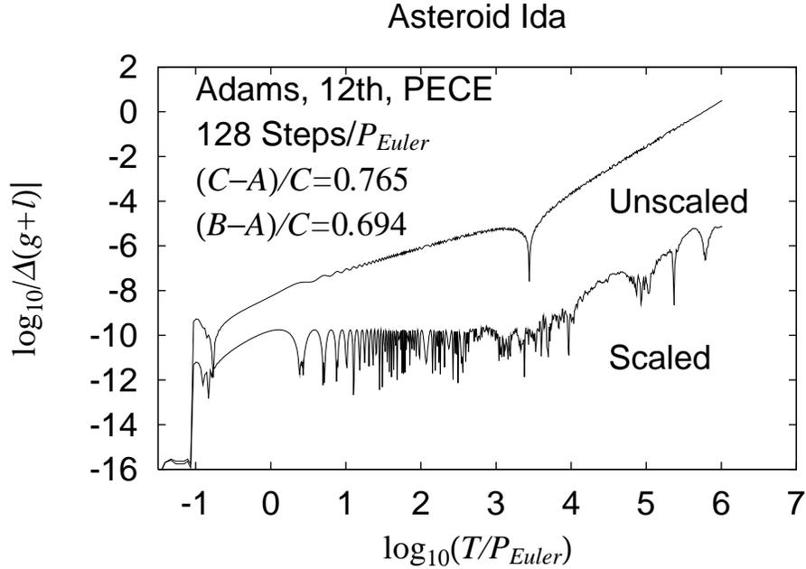
Figure 3: Same as Figure 1 but for the asteroid Ida. The initial angle  $J_0$  was taken as relatively large 0.1 radian. The chosen step size was 1/128 of its Eulerian period.
