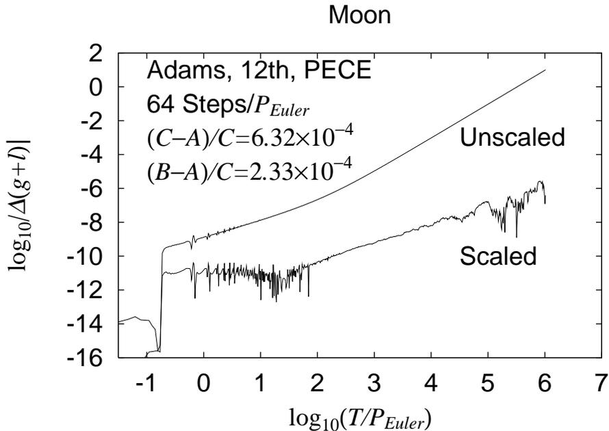
Figure 2: Same as Figure 1 but for the torque-free rotation of a rigid Moon. The initial angle  $J_0$  was taken as  $10^{-5}$  radian. The chosen step size was relatively small as  $1/64$  of its Eulerian period.
