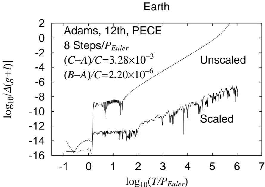
Figure 1: The numerical integration errors in the combined rotational angles  $g + \ell$  of the torque-free rotation of a rigid triaxial Earth are shown as functions of time in a log-log scale. The initial angle of inclination,  $J_0$ , is chosen as small as  $10^{-6}$  radian. The step size was as large as  $1/8$  of the Eulerian period,  $\sim 300$  days.
