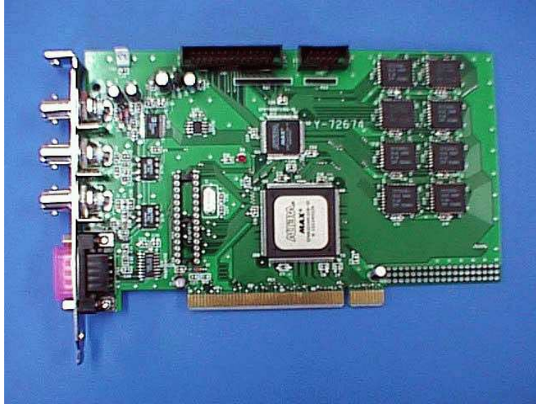
Figure 2: A PCI sampler board for the IP-VLBI system.
