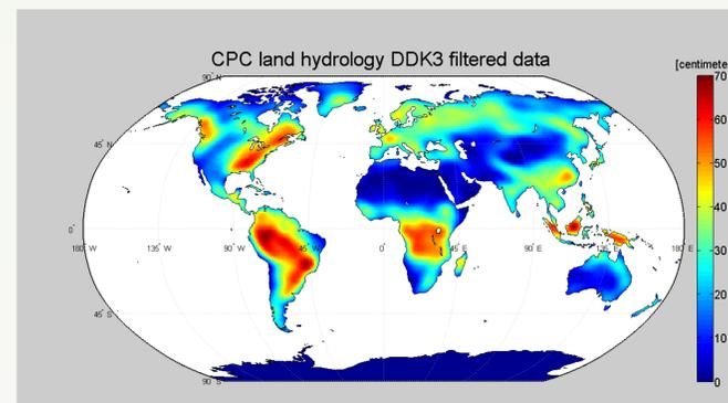
Figure 2b): EWT map from CPC model from January 2007 with usage of DDK3 filter
