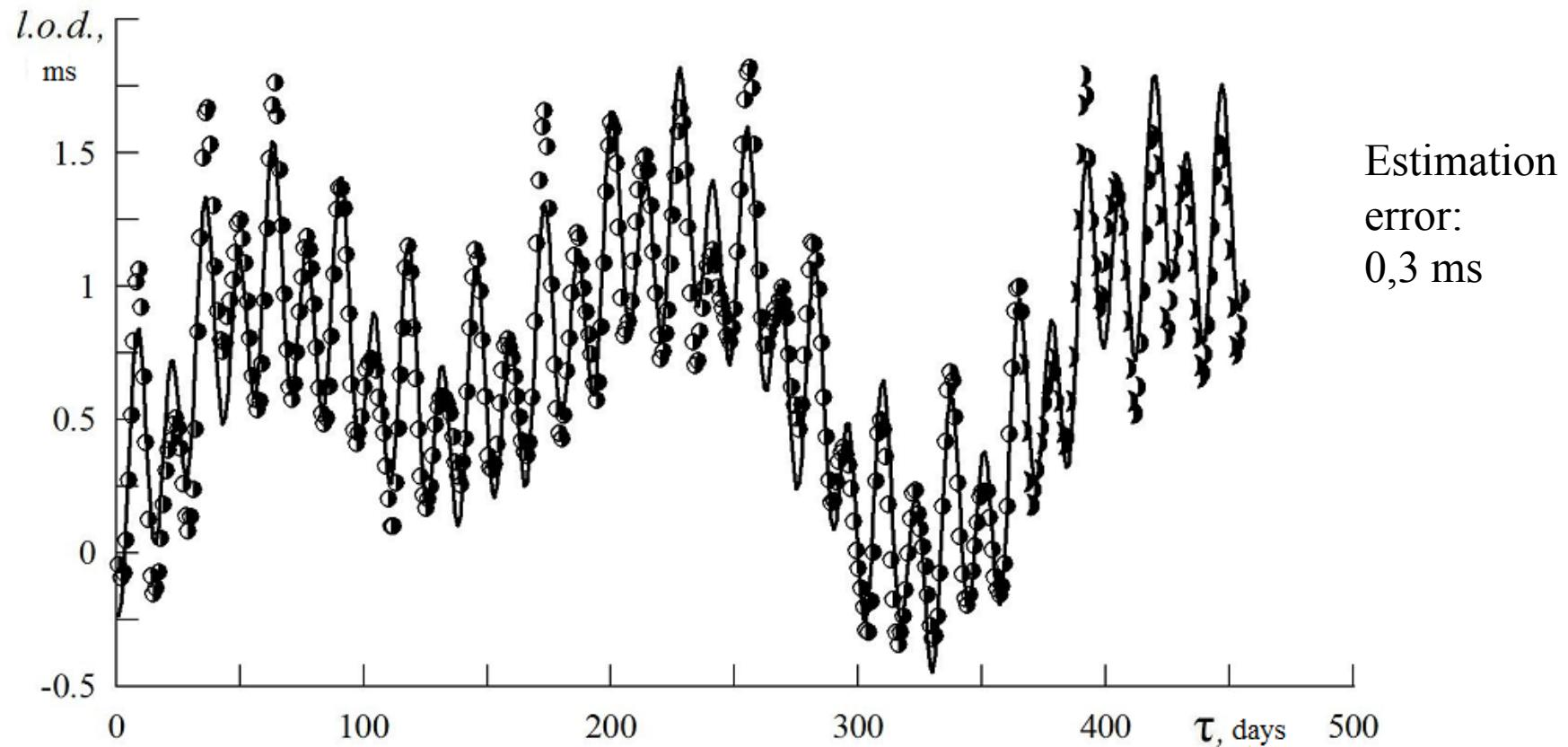
Interpolation (September 2010 - September 2011) and forecast (September 2011 - January 2012) of l.o.d. Solid curve – theoretical model, dots are IERS observation data
