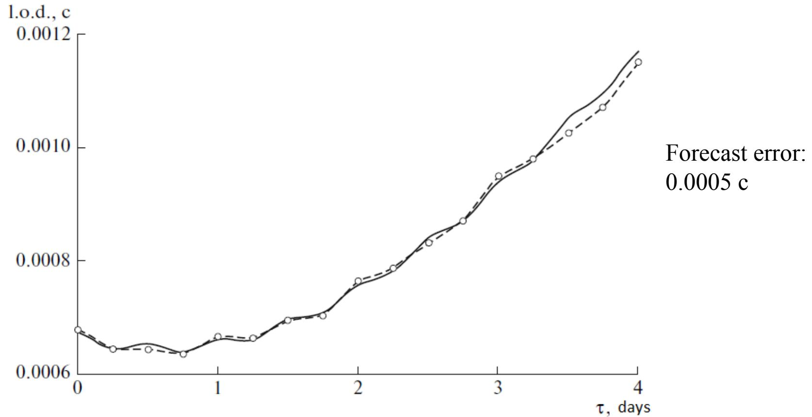
Interpolation (2.5 days) and forecast (1.5 days) diurnal oscillations of the l.o.d. ( $\varphi, \tau$ ). Solid curve – theoretical model, dash-dots – observations data
