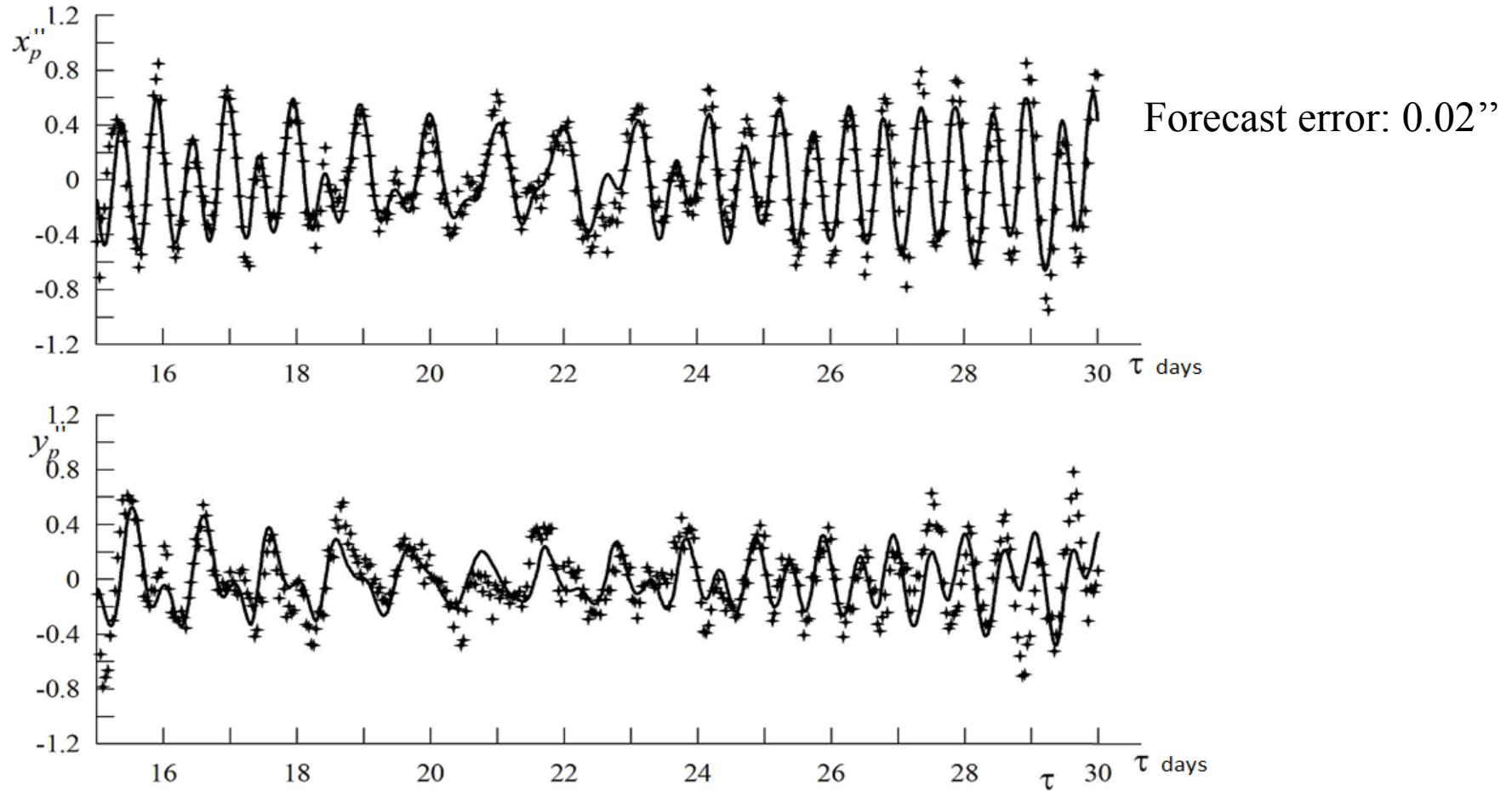
Interpolation of the subdiurnal oscillations for  $x_p$  and  $y_p$  of the Earth's pole from 15.09.2011 to 27.09.2011 and forecast for 3 days (solid curve) in comparison with VLBI data (stars).
