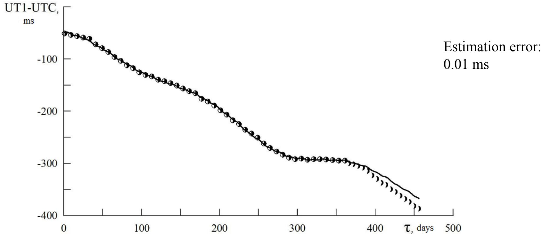
UT1-UTC interpolation (September 2010 - September 2011) and forecast (September 2011 - January 2012) of UT1-UTC. Solid curve – theoretical model, dots are IERS observation data.
