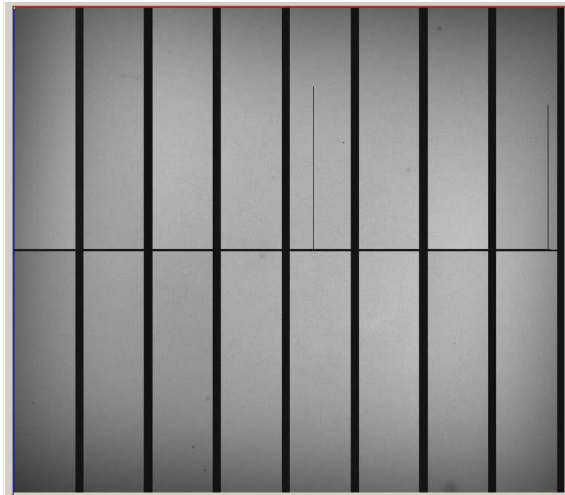
Figure 4: Flat field image of a successfully thinned 10k detector for the URAT camera. Pixel data of the 16 outputs are shown with overscans. The cosmetic quality is excellent with only 2 column defects on the entire 111 million pixel area.
