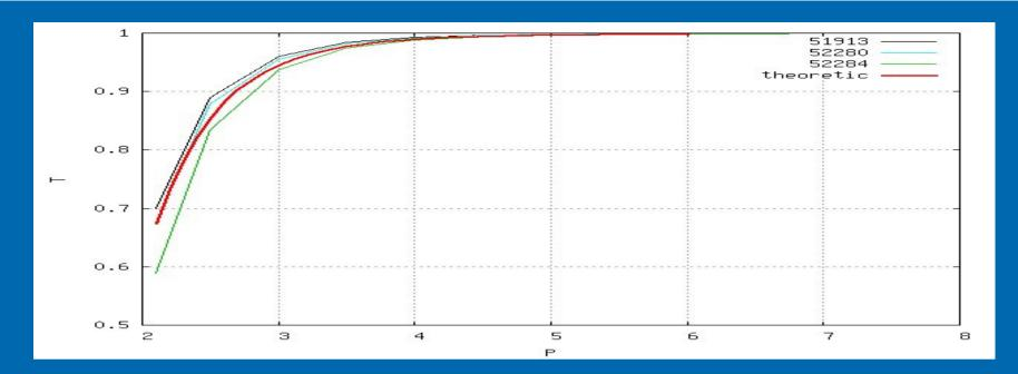
$\succ$  This graph shows comparison of computed transfer function with theoretic one.
