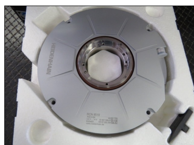
Figure 5: New HEIDENHAIN 26-bit absolute angle encoder. Credit: P. Mey.
