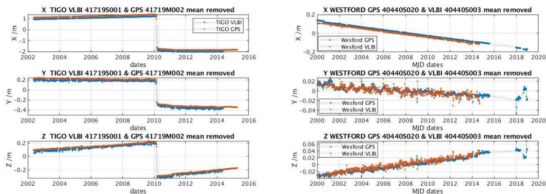
Figure 6: X, Y, Z displacements of GPS/VLBI collocated stations of TIGO and Westford
