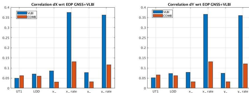
Figure 5: Correlations between nutation offsets  $dX$  and  $dY$  with the others EOP, VLBI only and combined solution (COMB)
